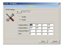
This window allows the user to configure the Print Server to automatically get its IP address from the network's DHCP server, or manually specify a static print server IP address. The Print Server also has a built-in DHCP server that manages the Print Server IP addresses.
